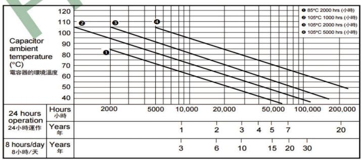
Example: When a 2000 hours/105°C guaranteed product is used continuously at 60°C, it can be expected to have a life of 5 years.
